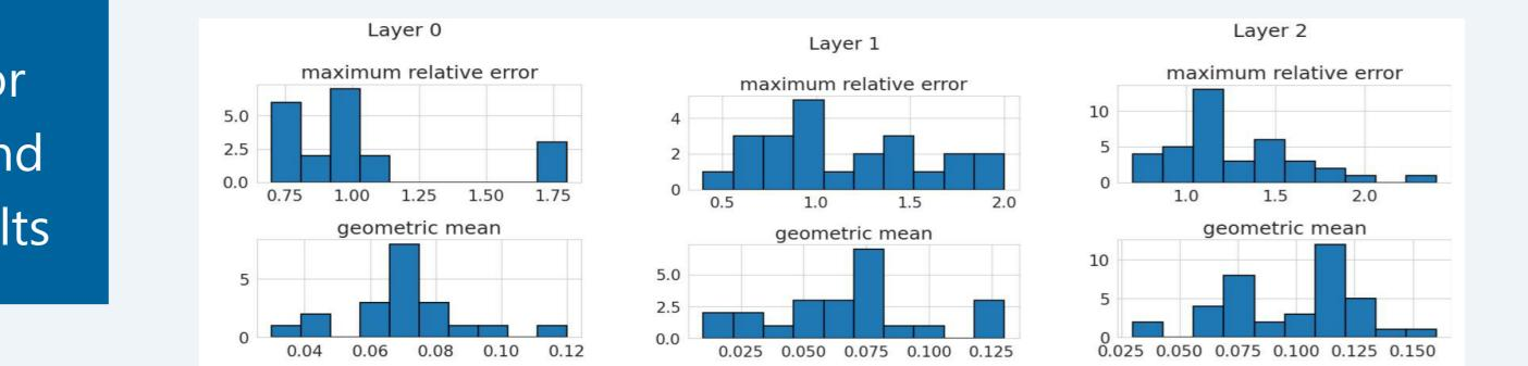
Error of the neurons on the **test-set** of an MNIST network with 3x100 neurons, reduced by 30%.
